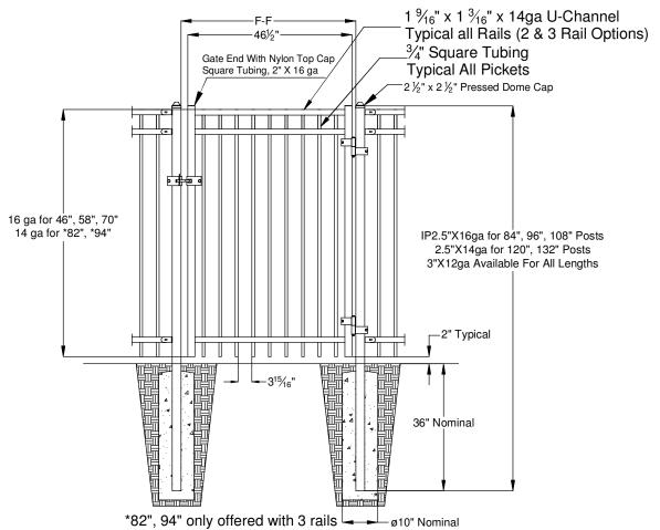
F-F: TYPICAL SPACING 49  $\frac{1}{2}$ "POST FACE TO POST FACE . SPACING CAN VARY DEPENDING ON GATE HARDWARE USED. CONSULT GATE HARDWARE INSTRUCTIONS. VERSAI RINGS-3D-RES
