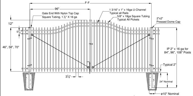
F-F: TYPICAL SPACING FOR TWO 08 DDGP-196  $\frac{1}{2}$ " SPACING CAN VARY DEPENDING ON GATE HARDWARE USED. CONSULT GATE HARDWARE INSTRUCTIONS.
