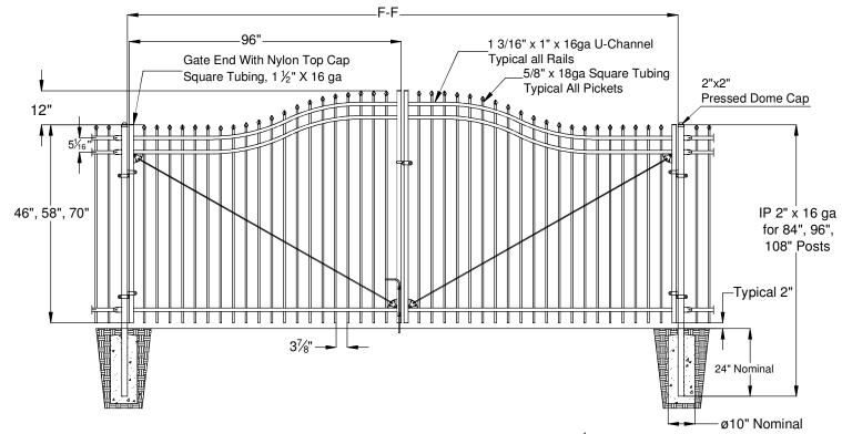
F-F: TYPICAL SPACING FOR TWO 08 DDGP-196  $\frac{1}{2}$ " SPACING CAN VARY DEPENDING ON GATE HARDWARE USED. CONSULT GATE HARDWARE INSTRUCTIONS.
