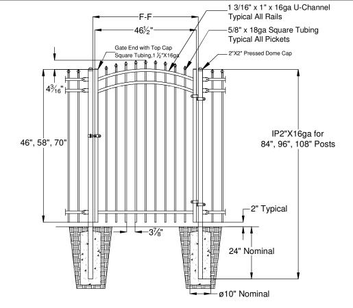
F-F: TYPICAL SPACING 48  $\frac{1}{2}$  "POST FACE TO POST FACE . SPACING CAN VARY DEPENDING ON GATE HARDWARE USED. CONSULT GATE HARDWARE INSTRUCTIONS.
